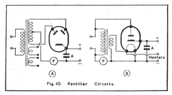
Valuable protection to the rectifier and transformer can be given by inserting simple fuses in the circuit as shown in Fig. 10. They can be of the flash lamp bulb type, with a current rating to suit the load to be taken from the power pack with extra provision for any surges that might occur as the condenser charges up.
